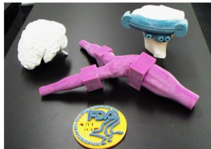
3D printed (left to right, top) models of a brain, blood vessel, surgical guide, and (bottom) medallion printed on FDA 3D printers.
